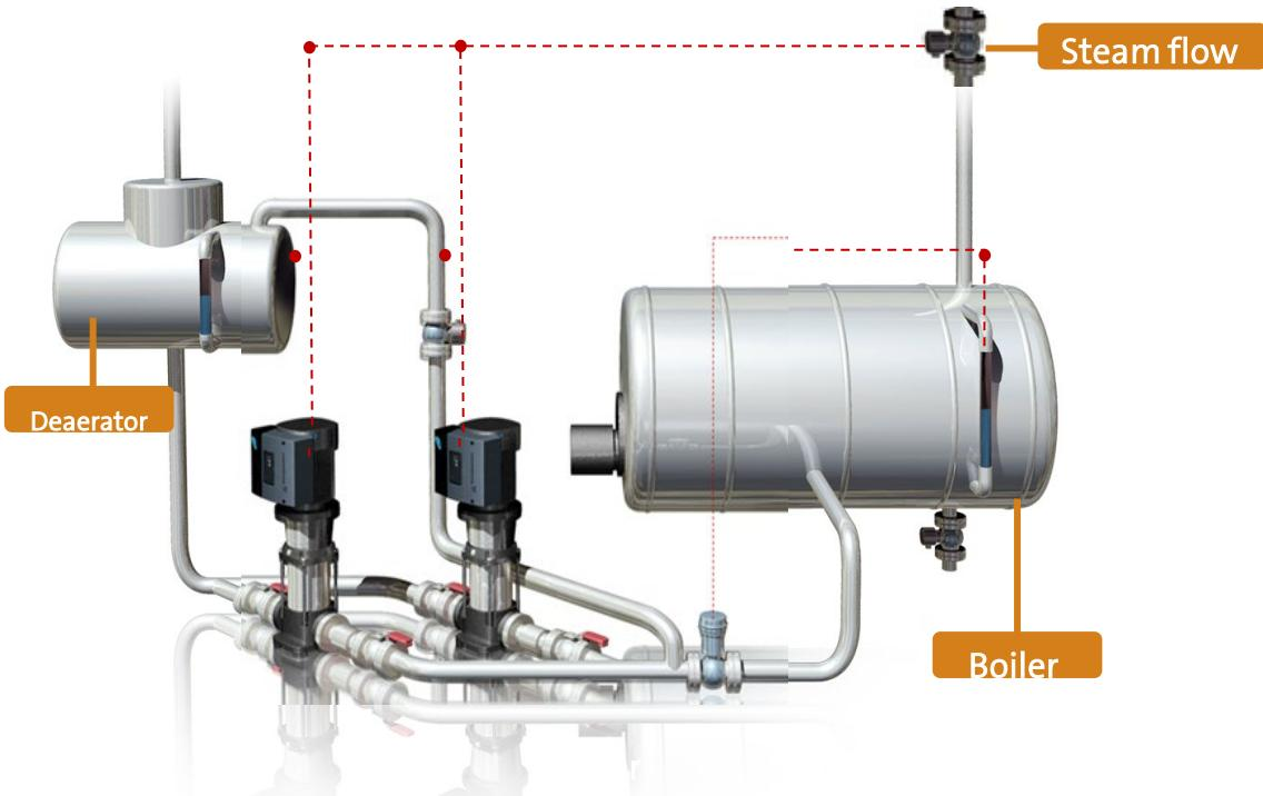
**The Setpoint Influence Function-** Allows the pump to readjust the Setpoint based on the monitored input signal (sensors). It is most suitable for application which has multiple fluctuation of input signal (sensors).
