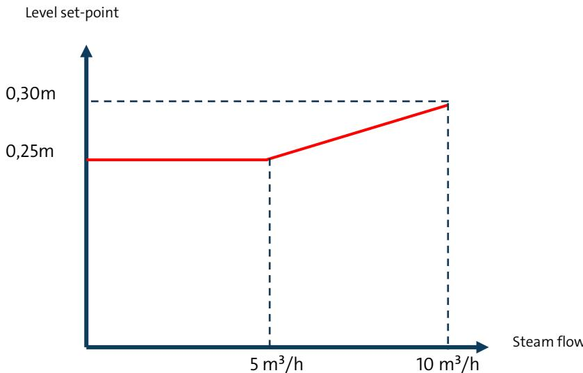
**Example:** Water Level is 0.25m when steam output is 5m<sup>3</sup>/h. When it increases to 10m<sup>3</sup>/h, then the setpoint will auto readjust the Water Level to 0.30m. This is to avoid the increase of start-stop for the pump when the boiler burn faster than the incoming water into the tank.
