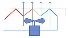
Dry coolers are used either as a free cooler or to cool the condenser in a refrigeration system.
