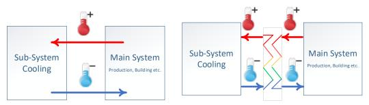
Cooling and/or refrigeration will in some form be present in almost every industrial production or process facility. The purpose of industrial cooling is to cool and remove heat from industrial machines, such as welding and injecting moulding machines, as well as industrial processes, including dairy, chemical and fermentation.
