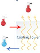
A cooling tower is a heat rejection device that ejects waste heat to the atmosphere by using ambient air to cool water to a lower temperature. Cooling towers either use the evaporation of water (evaporative cooling towers) to remove process heat and cool the working fluid to near the wet-bulb air temperature, or by using ambient air (dry cooling towers). This relies solely on air to cool the working fluid to near the drybulb air temperature.
