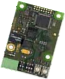
Grundfos Communication Interface Modules (CIM) enable communication via all relevant fieldbuses.
