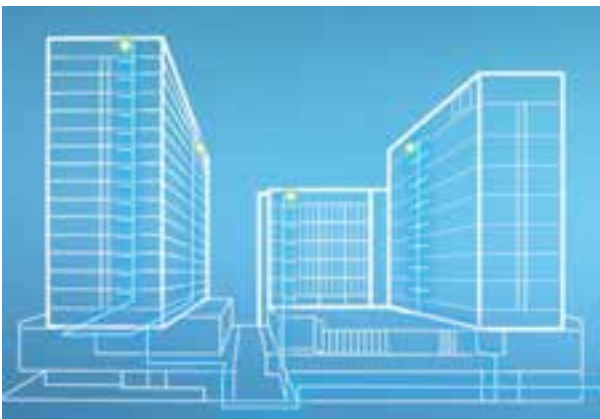
An example of a commercial building with a widespread water system. It can be challenging to determine the critical point, so up to six pressure sensors will be enough to cover the entire system.
