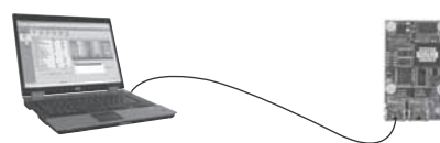
Fig. 20 CIM 500 connected to a PC via Ethernet cable
