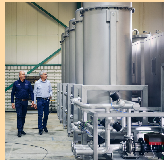
John and Freddy at the reactor vessels where the oxidation takes place.
